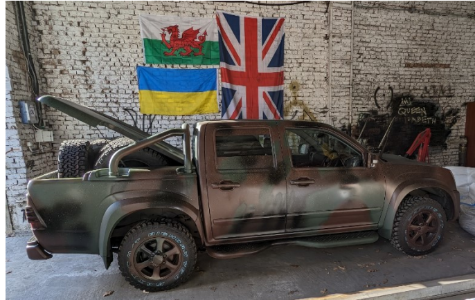
3 Resprayed and fitted with mud tyres ready for active medical service
